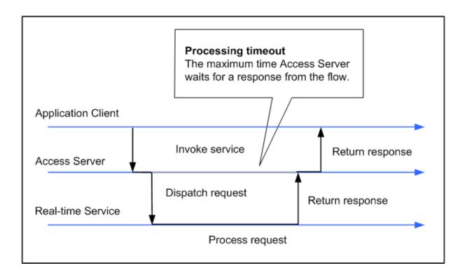
If *Processing retry count max* is set to zero, the maximum response time is equal to the queuing timeout plus the processing timeout.
