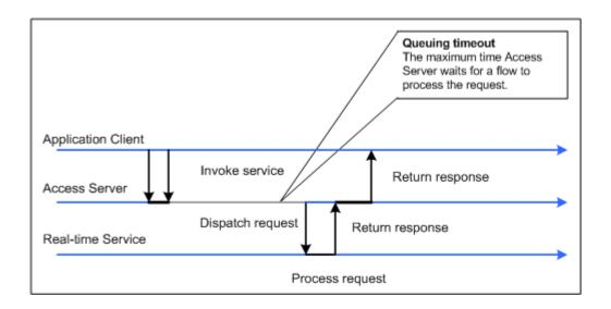
A service experiences high traffic when the available resources cannot process the received requests efficiently. High traffic occurs when the time messages wait to be processed exceeds the time required to process them.
