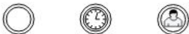
The event listener, timer event listener and user event listener elements (left to right)
